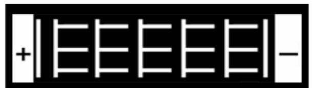
**WARNING!** Do not connect a charged battery backwards or reverse polarity to the solar module, this will destroy the solar module and may cause the battery to explode.
